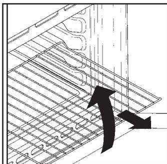
The oven features a new shelf safety system. This allows you to pull out the oven shelves when inspecting the food without danger of food spillages or shelves falling accidentally out of the oven. To remove the shelves pull out and lift.
