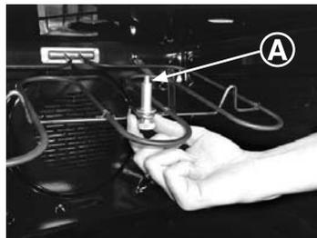
For routine cleaning access can be gained to the upper parts of the oven by removing the screw and washer (A) from the middle of the grill element and then gently tilting the element in a downward direction. Once cleaned the grill can be returned to the correct position by reversing the above procedure.
